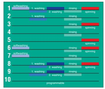
Nine different washing cycles: just choose one and press the button! On the inside of the lid you'll find information about which program to use: be it the rinsing program which cleans by gently moving the water or by using the variable water jets for more heavily soiled produce. You can follow the program on the display.
