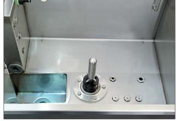
This is what hygiene really looks like: stainless steel inside, rounded corners and edges, water jets at the bottom and at the sides, also made out of stainless steel. Everything is easily accessible, no need for special tools if you want to take it apart for thorough cleaning.
